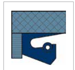
Model 161-0 Universal Oil Seal 161-0 is available in an endless version only, with PTFE backup ring.*
