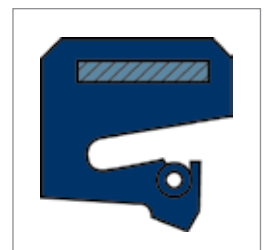
Model 154-M Universal Oil Seal 154-M incorporates a metallic reinforcement ring molded into the heel and can be installed without a cover plate.
